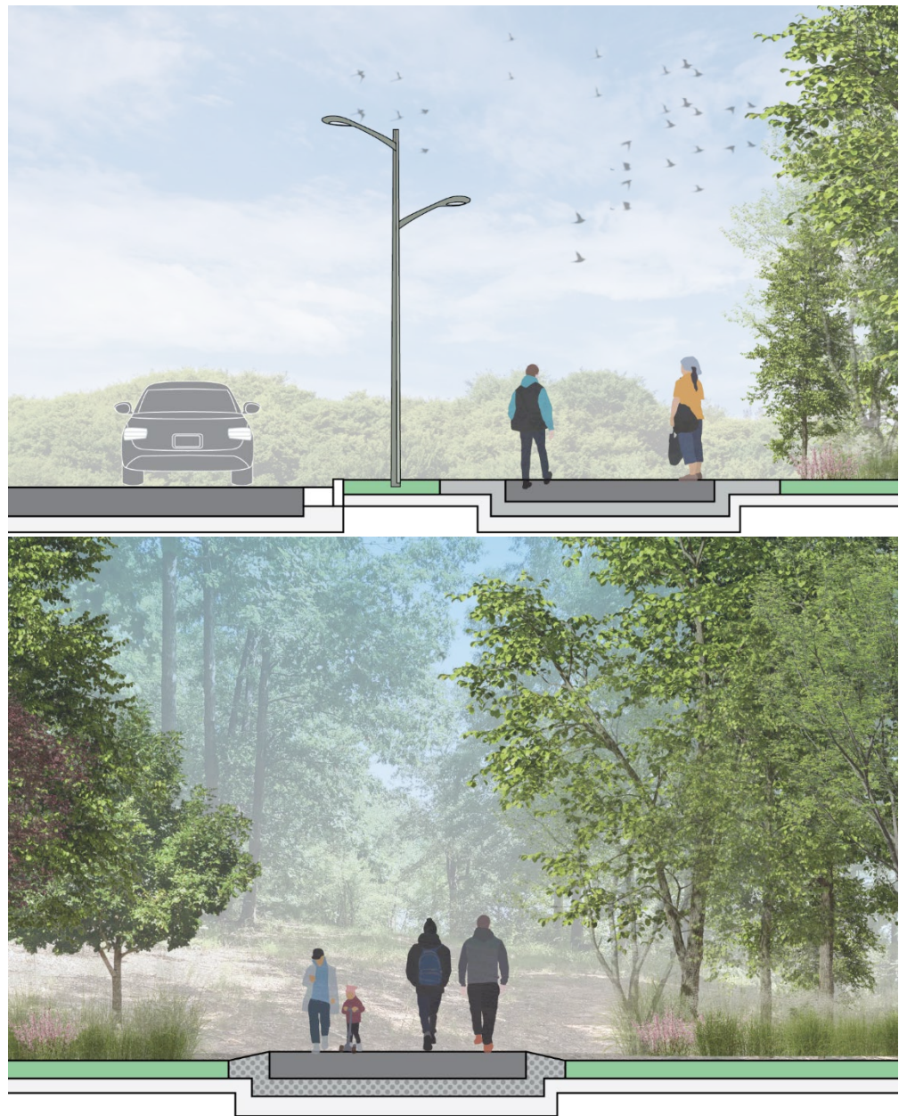
Figure 11. Typical Shared Use Path Cross-Section through a Wooded Area (Bottom) and Along a Roadway (Top)
